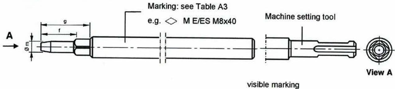
**Verification of correct installation with setting tool for marking**
