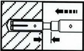
Drive in cone by using setting tool.
