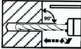
Drill hole perpendicular to concrete surface.
